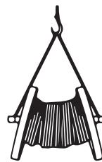
Avoid damaging or lateral on flanges while being hoisted.
