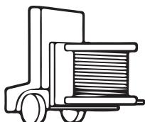
Carefully insert forklift into pallet and/or lifted on both flanges.
